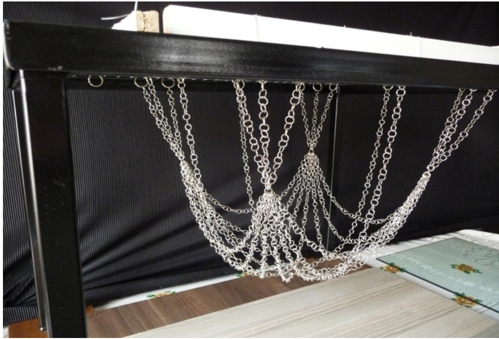
Figure 4.36: Physical model with broad corner and centre supports
