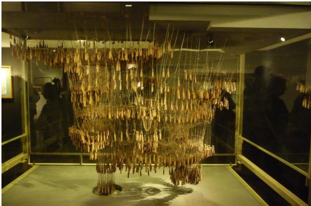
Figure 2.6: Gaudi's string model with birdshot weights used in the design of the Colonia Guell.
