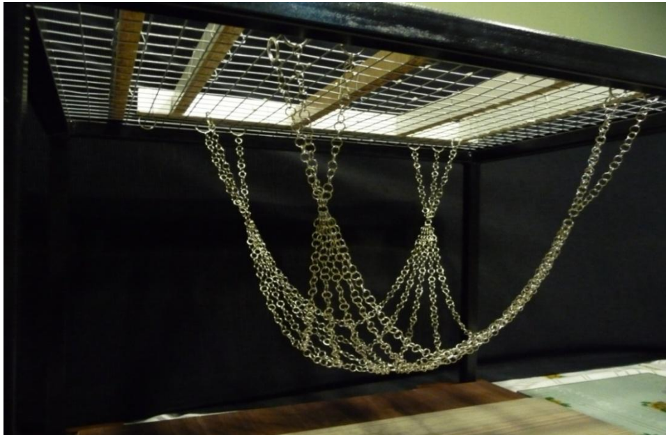
Figure 4.28: Physical model with broad corner supports
