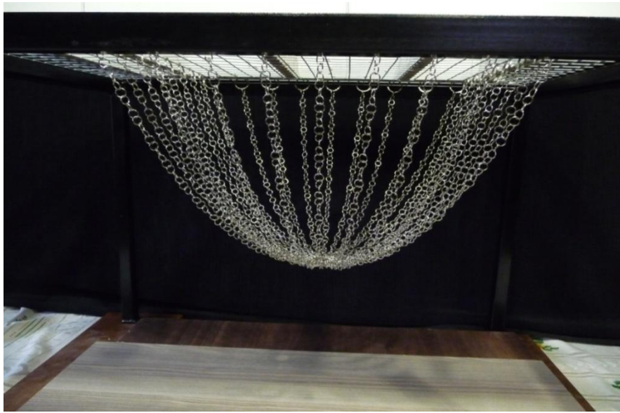
Figure 4.12: Physical model with all edges simply supported
