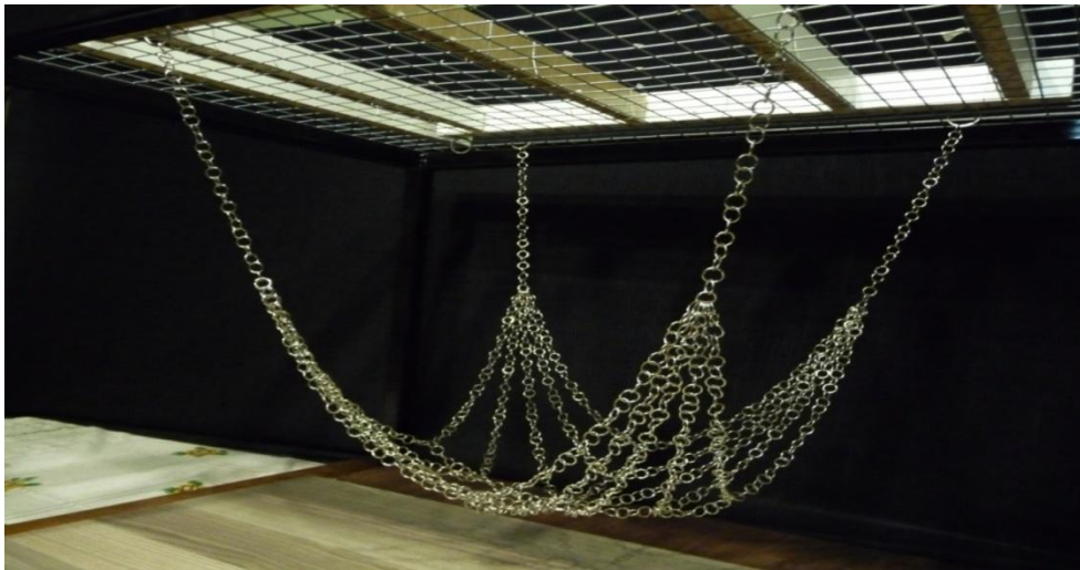
Figure 4.20: Physical model with corner point supports
