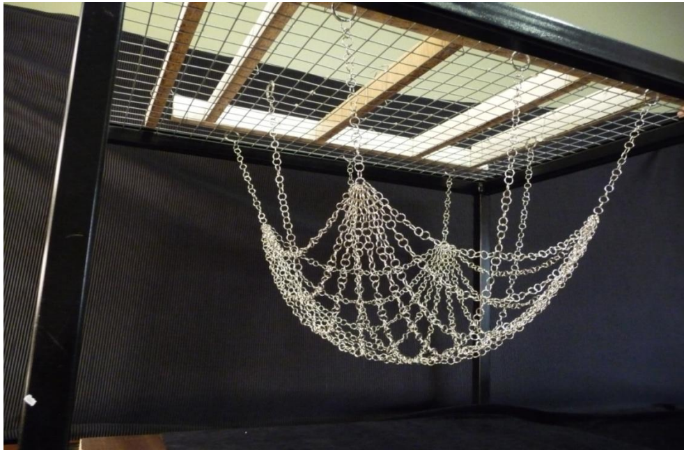
Figure 4.44: Physical model with corner and centre point supports
