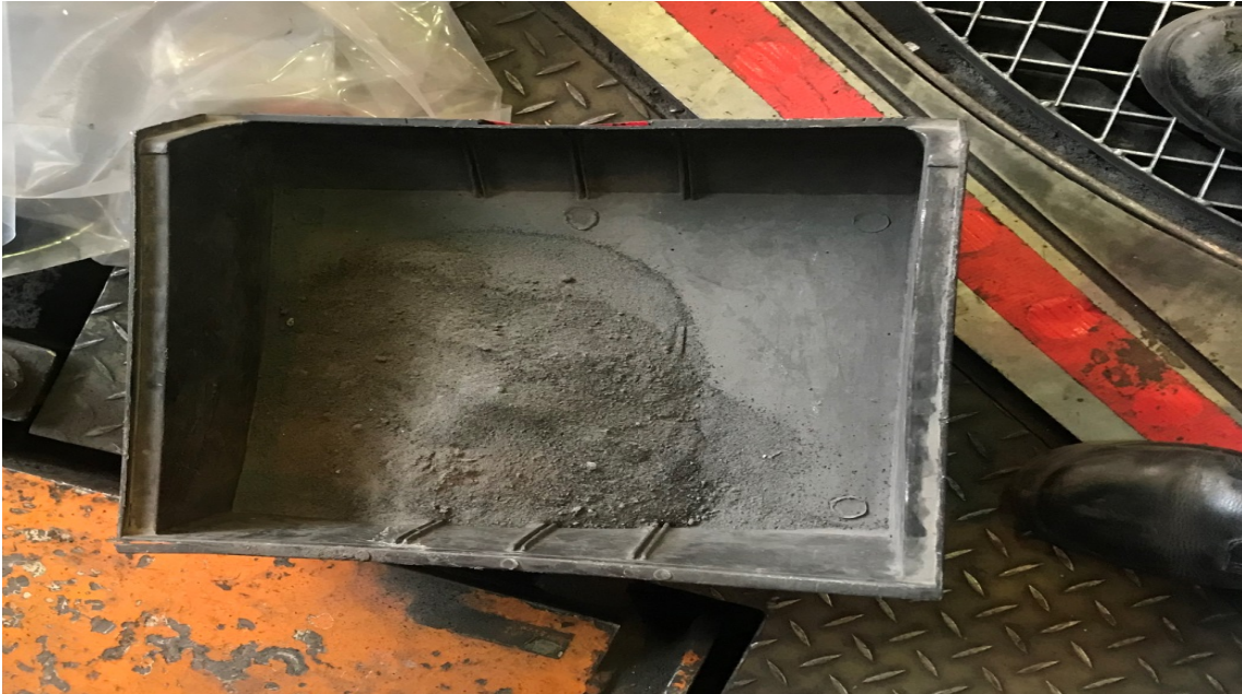
Figure 50: Grit taken out from one of the bearing pedestals in the unit.
