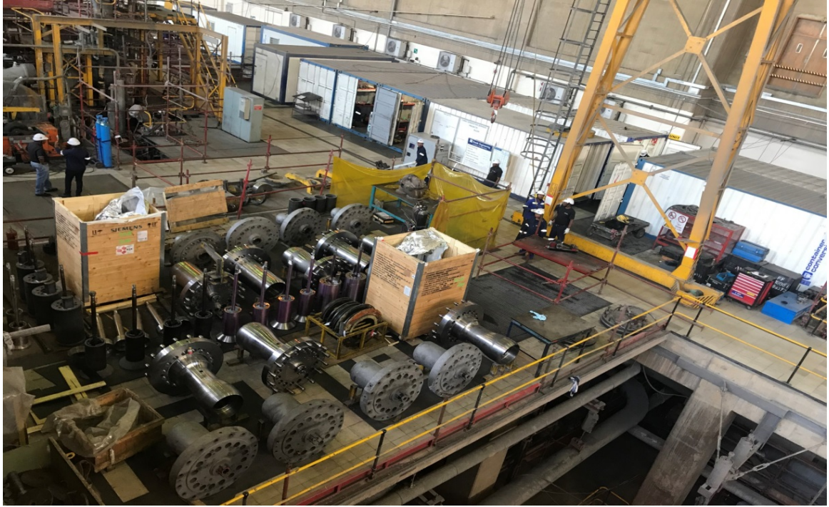
Figure 48: Containers placed in ‘heavy duty areas’ where heavy components could have been placed; and valve components stored next to the unit.
