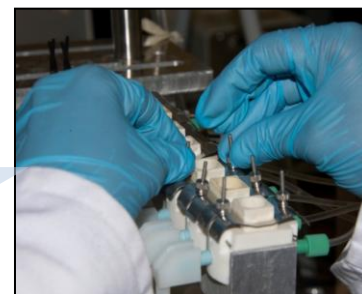
Holding donor chambers with a clamp
