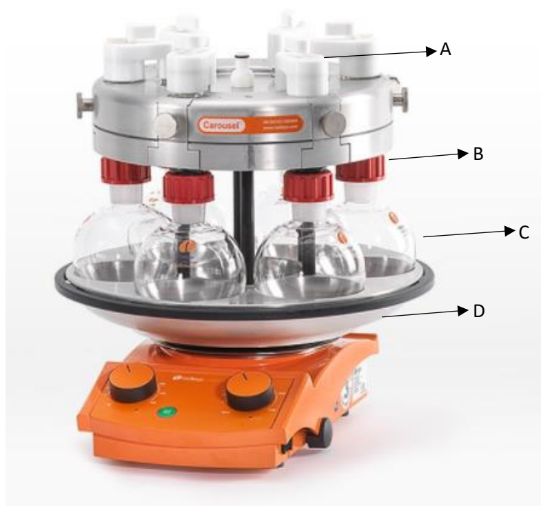
Figure 3.6: 6-vessel reactor where A. rubber seal, B. PTFE cap, C. round bottom flask, and D. Stirring hot plate.
