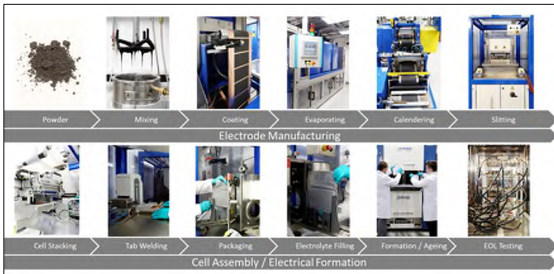
Figure 9: Li-ion batteries cell production process.
