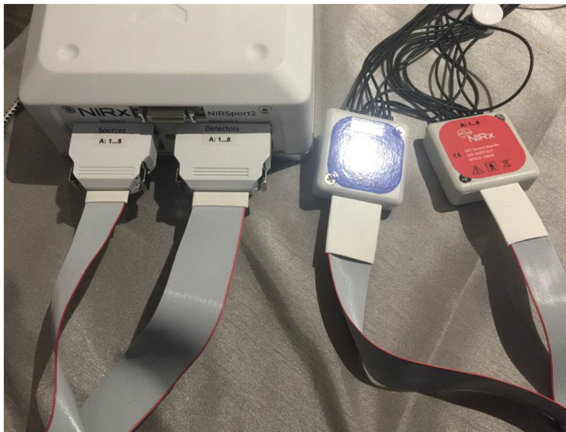
Fig. 11. NIRxSport2 correct source (red) and detector (blue) placement. (For interpretation of the references to color in this figure legend, the reader is referred to the web version of this article.)
