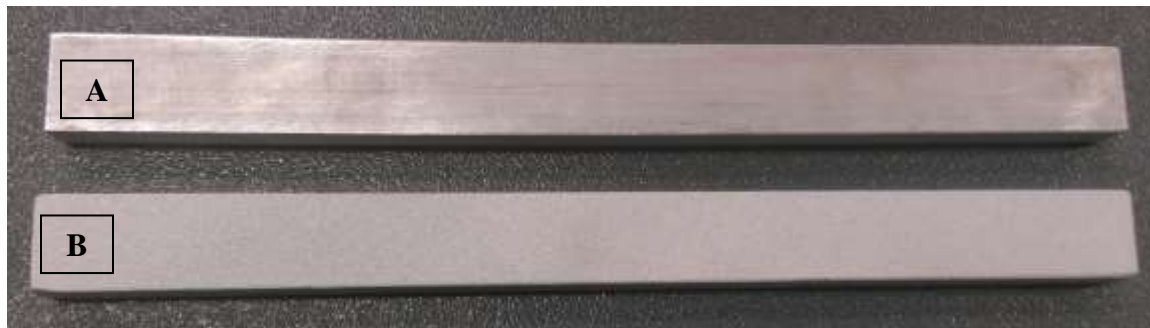
Figure 3.2: AA6082 strips of 240 mm length being prepared for plasma spraying.
