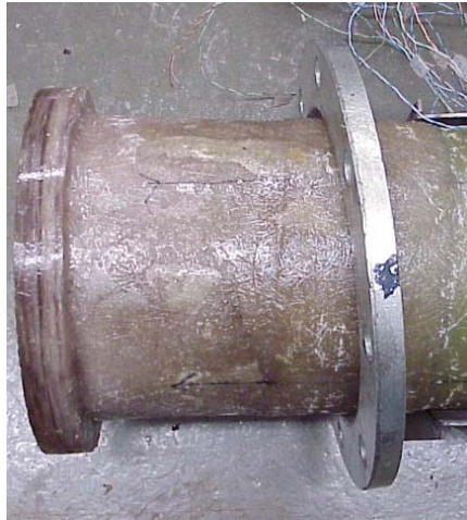
Figure 3.3: 10 bar fabricated flange
