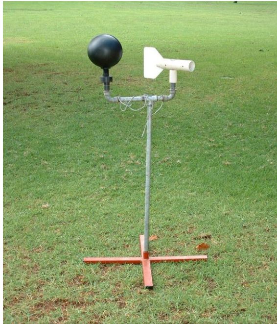
Figure 3.1: Weather station with black-globe temperature ( black copper ball ) and dry-bulb temperature ( white vane ) probes, positioned 1 m above ground in an open clearing.
