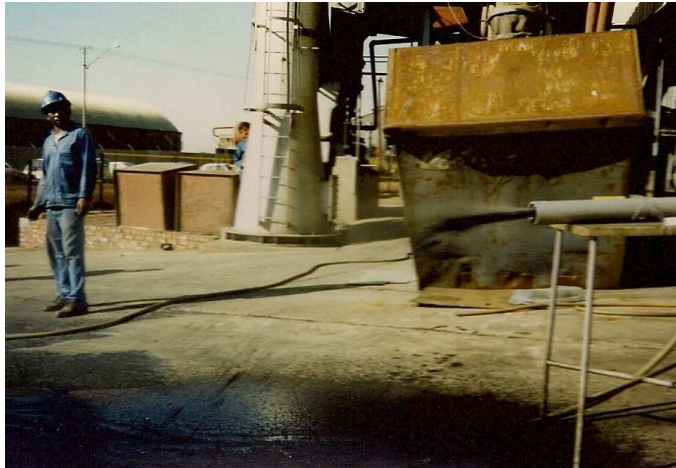
Figure 3.13 Coal slurry injection with full annular air
