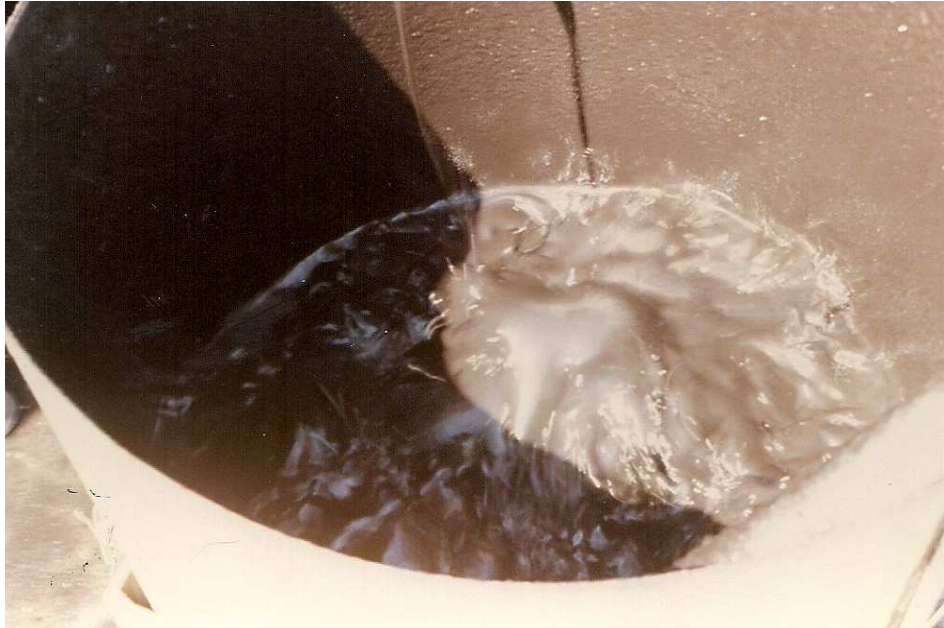
Figure 3.9 Coal slurry agitated by air injection in small tank
