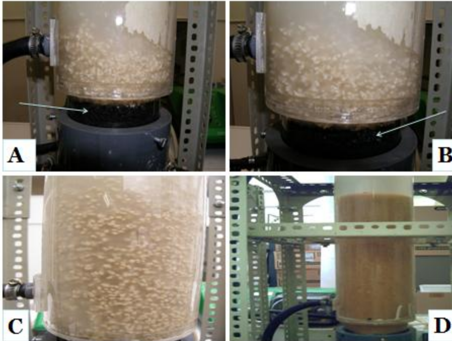
Figure 3.2: Different stages of AFGB system (A) AFGB column with activated carbon carrier ( CAC ) (B) CAC coated with bacterial flocs (biofilms) after granulation has been induced. (C) Expanded bed as a result of high organic loading rate, effluent degassed recycle rate and reduced HRT . (D) Settled bed
