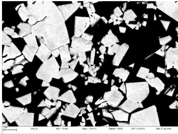
Figure 4.36. SEM image in backscattered electron mode of the corroded WC-30Co alloy showing no Co (holes (dark)) and WC (light).
