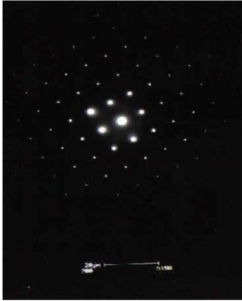
Figure 3.2. 10\bar{1} zone axis pattern from a WC grain in the WC-10VC-30Co alloy.
