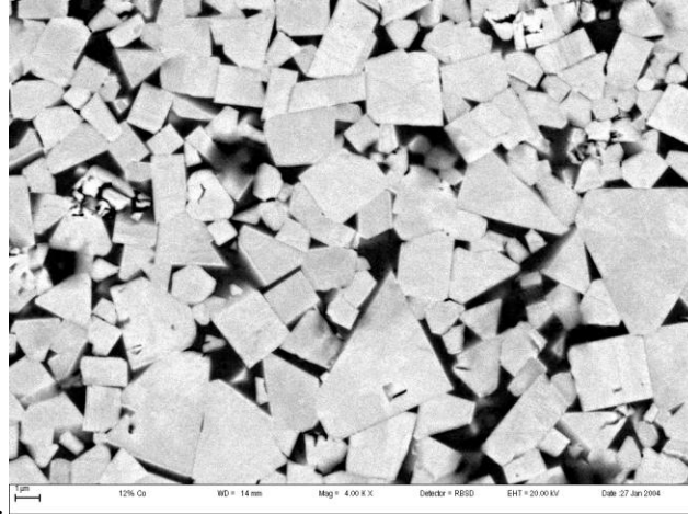
Figure 4.33. SEM image in backscattered electron mode of the corroded WC-12Co alloy, showing no Co (holes (dark)) and WC (light).
