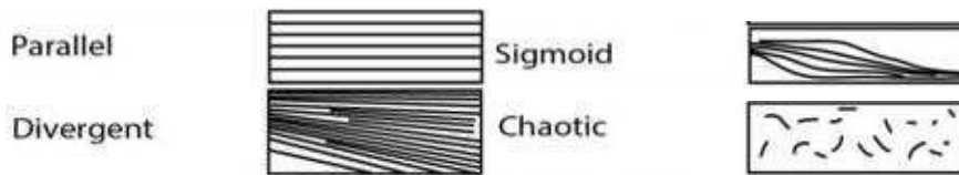
Figure 5.3: The four basic seismic reflection configurations (Papadimitriou, 2017).
