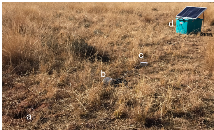
Figure 2.5: Field set up of the ACRS and power supply system. The antenna (a) is fitted over the burrow entrance, followed by placement of the reader board (b), then the cellphone engine (c) and the power box unit (d).
