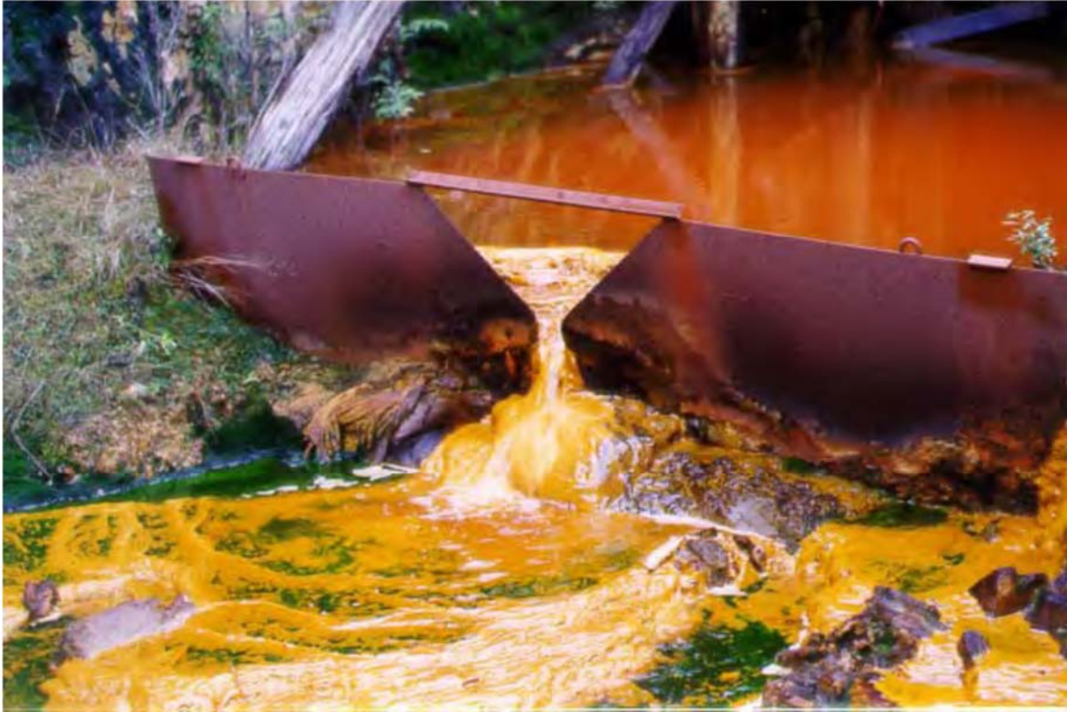
Figure 1.4: Acid mine drainage water from abandoned mine. The orange coloration is due to the iron (Fe) that has been mobilised by the sulfur oxidation process.
