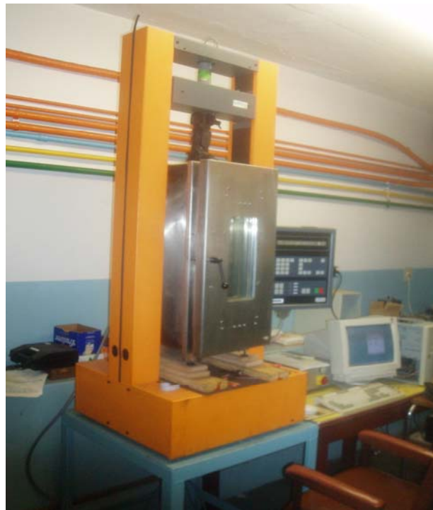
Figure 3.2 Lloyd machine with auxiliary components including a desktop computer and a control panel
