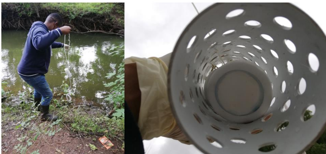
Figure 3.3. Field deployment of POCIS passive samplers (left), POCIS placed inside a cage (right) (Photograph: T. Letseka)
