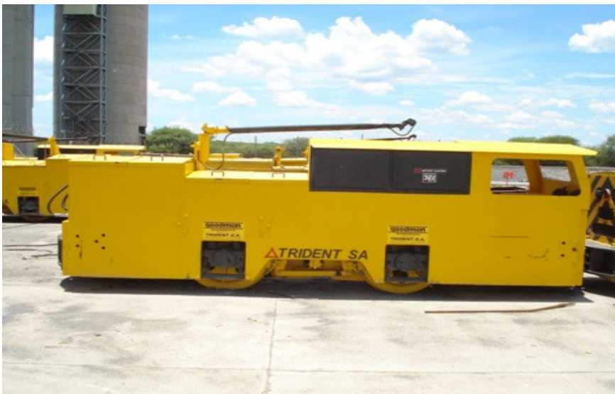
Figure 1. 10-Ton New Era locomotive currently used in the mining industry.
