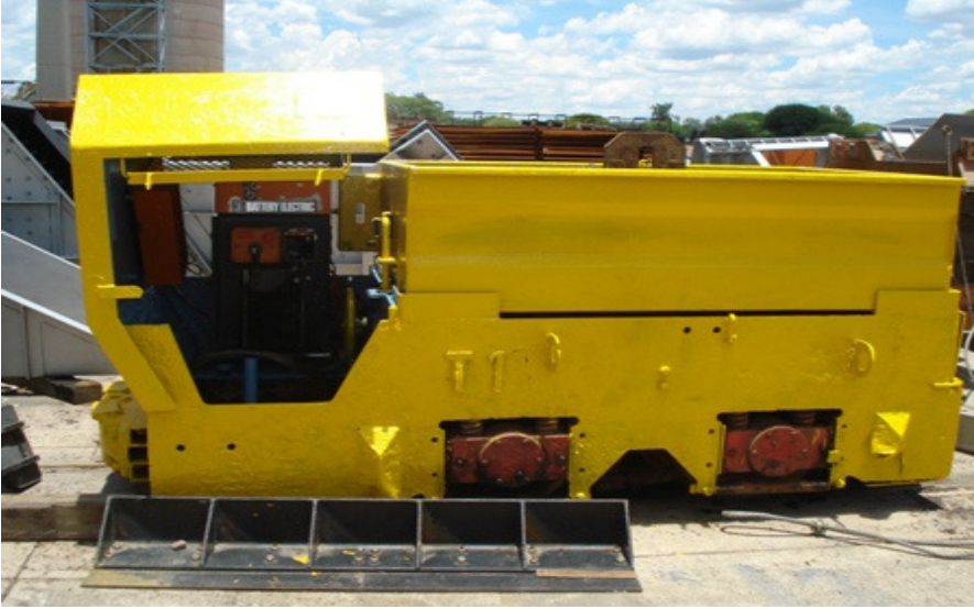
Figure 2. 10 Ton Goodman battery operated locomotive previously used in the mining industry.
