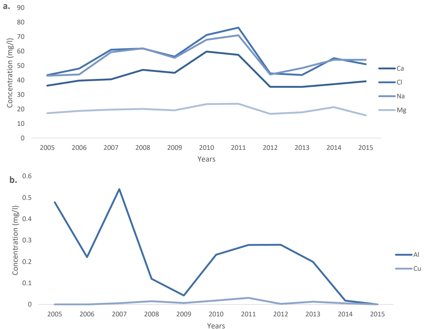
Figure 19. The averaged water quality data for all four rivers (Klip River, Hennops River, Blesbokspruit River and the Jukskei River) analysed by the Department of Water and Sanitation over the past 10 years (a. Calcium, Chlorine, Sodium and Magnesium; b. Aluminium and copper).
