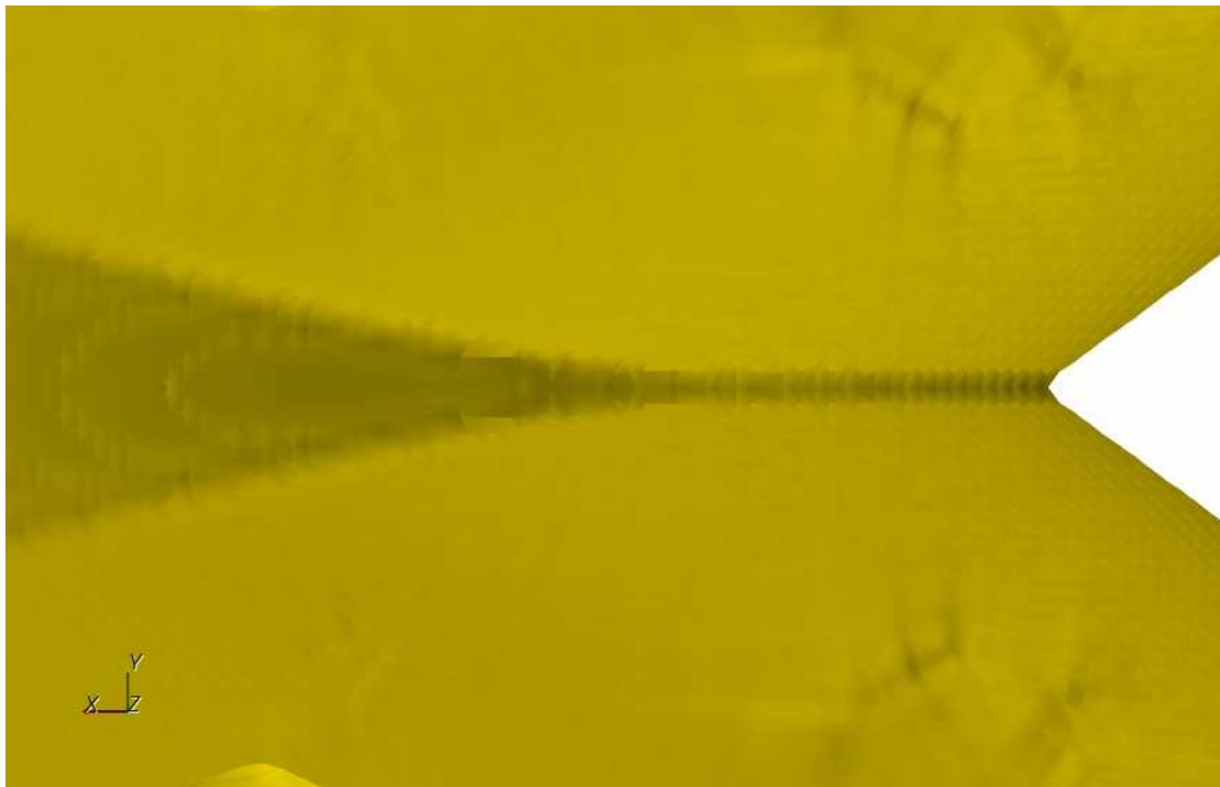
Figure 29: A close up of the transition from regular reflection to Mach reflection for figure 26.
