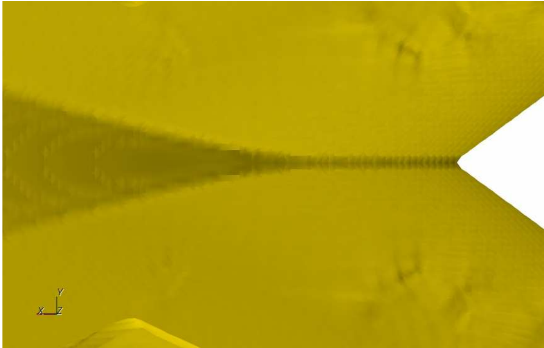
Figure 30: A close up of the transition from regular reflection to Mach reflection for figure 27.
