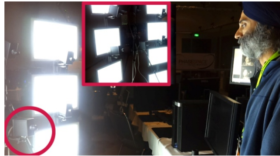
a) Kan Anant demonstrating the optimum position to stand before six high resolution cameras of the Phasespace Motion Capture System.
