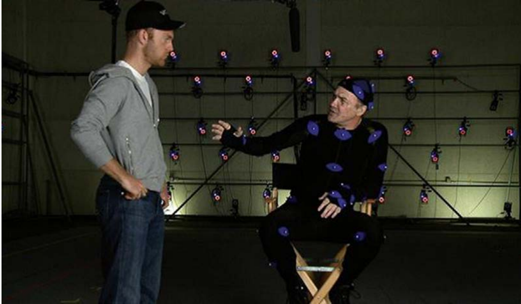
Fig 3: A performance in a typical optical, marker-based motion capture stage. In this picture, the cameras on the wall behind the performer have infrared lasers that catch the reflection from the marker or sensor. The term optical, marker based derives from the camera 'seeing' the marker on the suit. Source: Menache, Alberto. Understanding Motion Capture for Computer Animation (Second Edition) . Burlington, 2011. Print. 30 March 2013.
