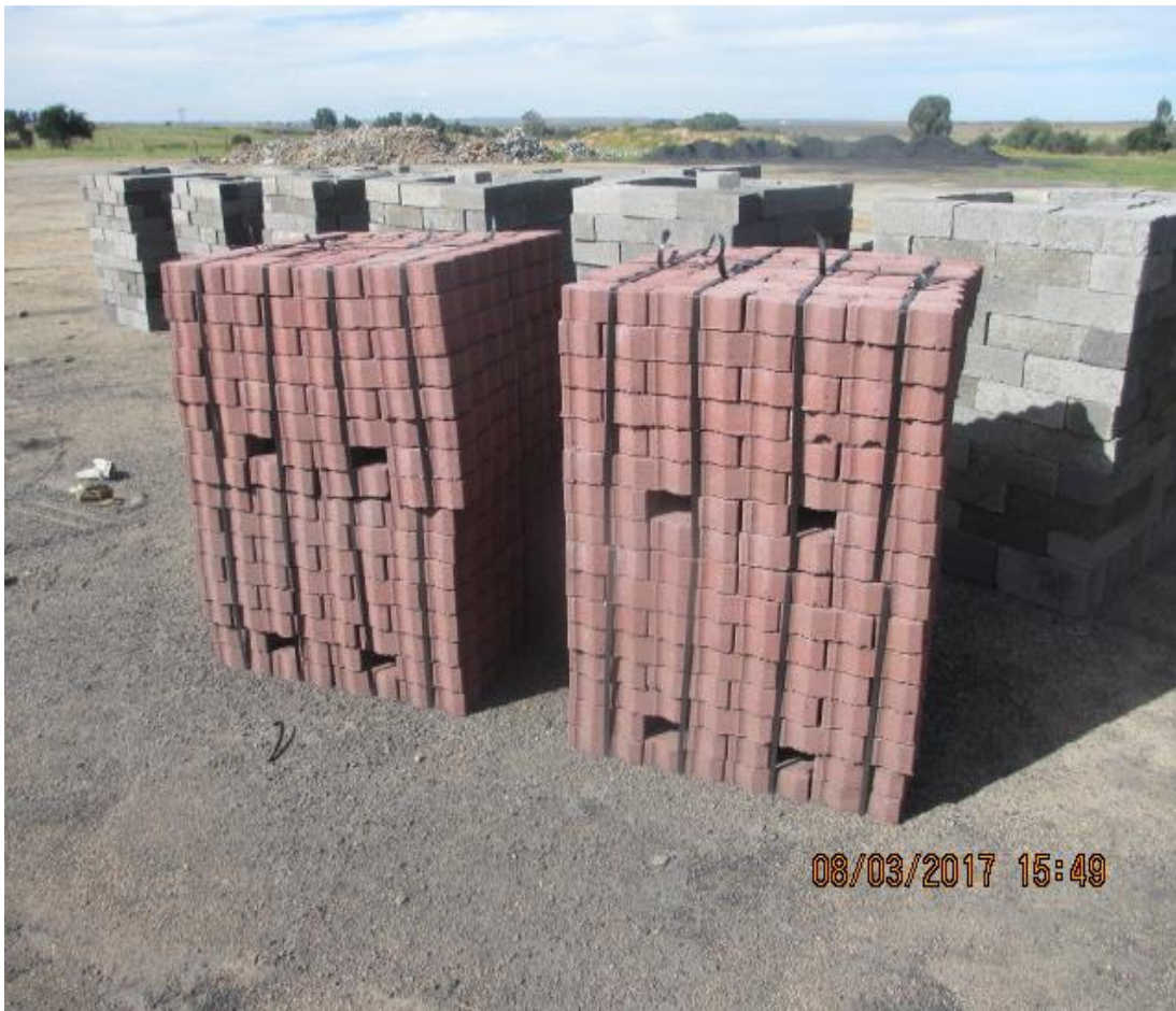
Photo 5: Bricks manufactured from course ash near Middleburg
