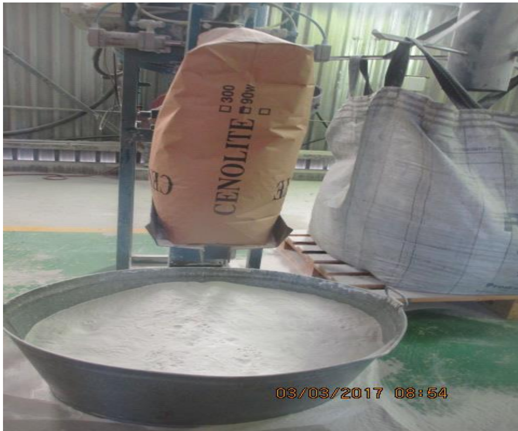
Photo 6: Collected cenospheres and processed to be Cenolite
