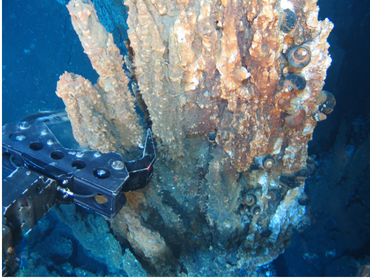
Figure 1.1: A robotic claw grasps a black smoker chimney. Image ©Nautilus Minerals Inc.
