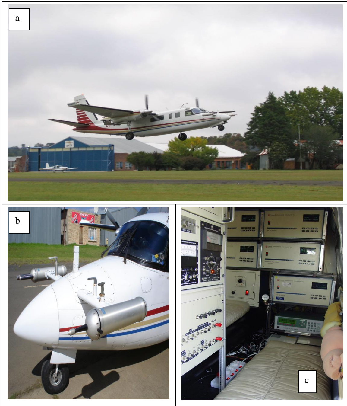
Figure 2.5: SAWS research aircraft and the research equipment on onboard. Figure 2.5(a) shows the aircraft taking off from Bethlehem airfield. Figure 2.5(b) shows the aerosol probes on the nose of the aircraft, the one on the left hand side of the aircraft is for fine particles and the one on the right hand side is for coarse particles. Figure 2.5(c) shows the data acquisition system and the trace gas instrumentation onboard.
