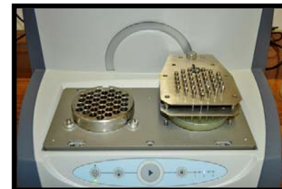
Figure 2.3: Flow Diagram illustrating the steps for inoculation of honey-agar plates and the multipointlite inoculator inoculating honey-agar plates.
