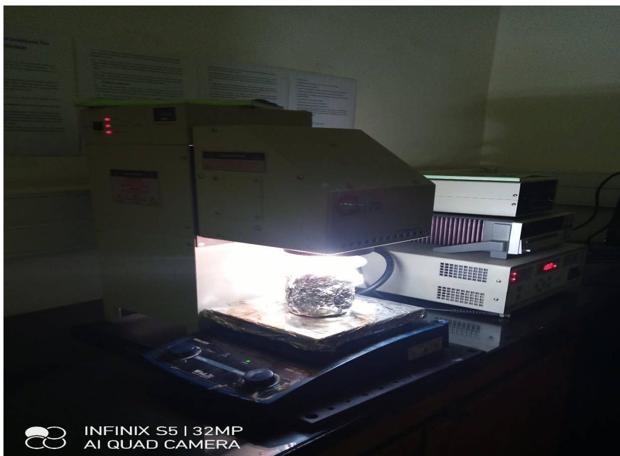
Figure 3. 6. AM 1.5G 100 mW/cm 2 Solar simulator
