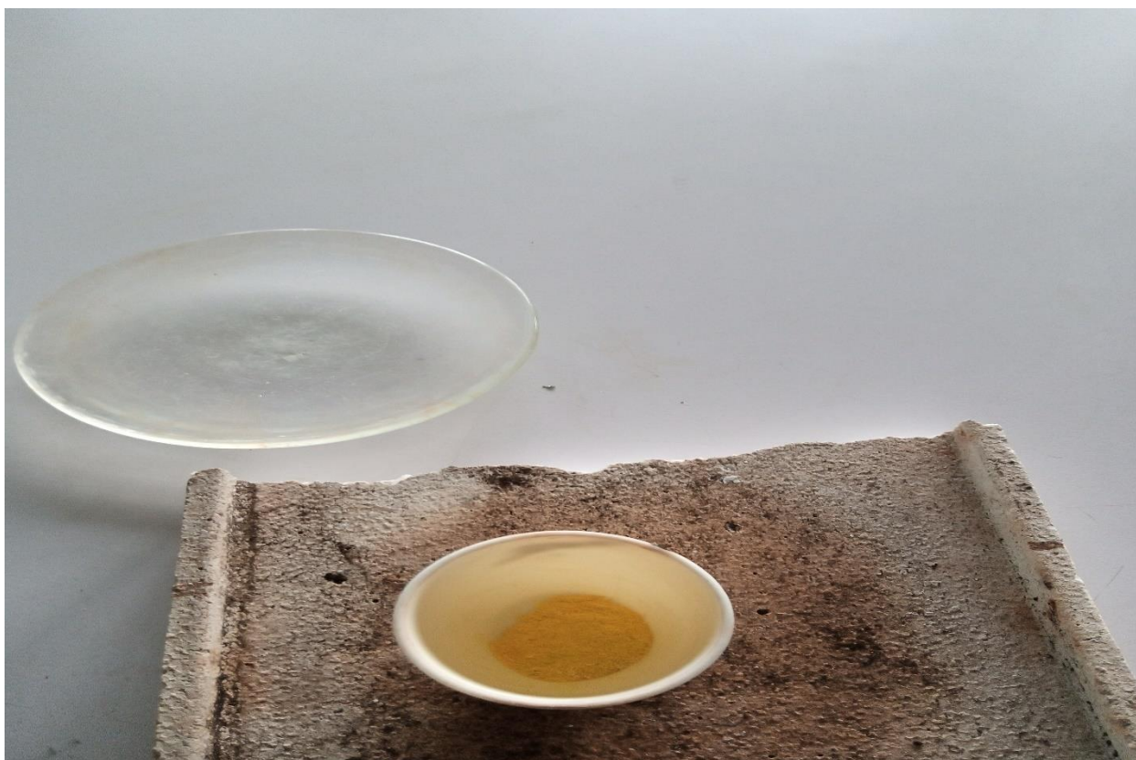
Figure 3. 2. WO 3 powder after calcination in furnace at 500°C for 2 hours.
