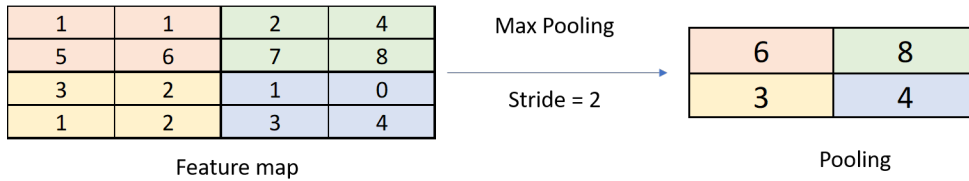
Figure 2.2: Example of Max pooling with stride 2
