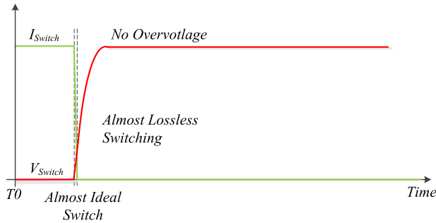
FIGURE 4. Voltage overshoot of optimised ZOS.
