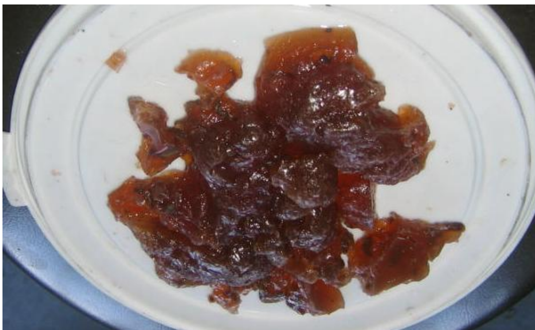
Figure 4.5: Lump formation as a result of acid over (2 M/ml) concentration
