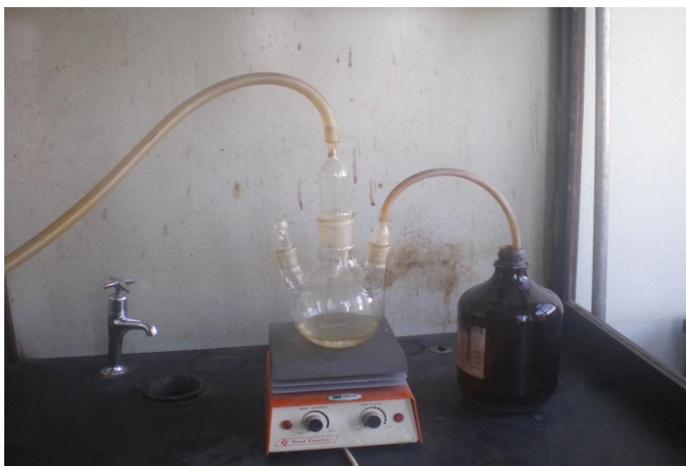
Figure 3.1: Experimental set up of chlorosulphonation of polystyrene-butadiene rubber
