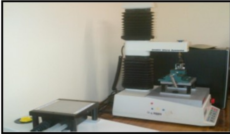
Figure 3.11: TA.XT Plus Texture Analyzer used for mechanical tests.
