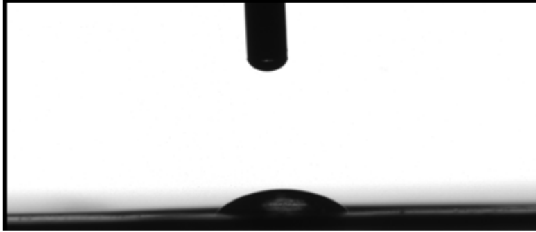
Figure 5.6: Illustration of the sessile drop measurement method [16]
