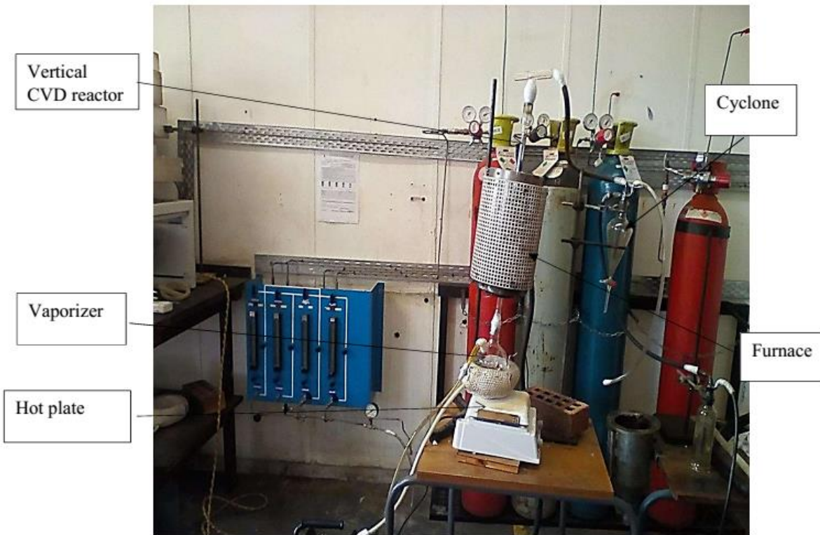
Figure 17: An experimental setup for CNT production
