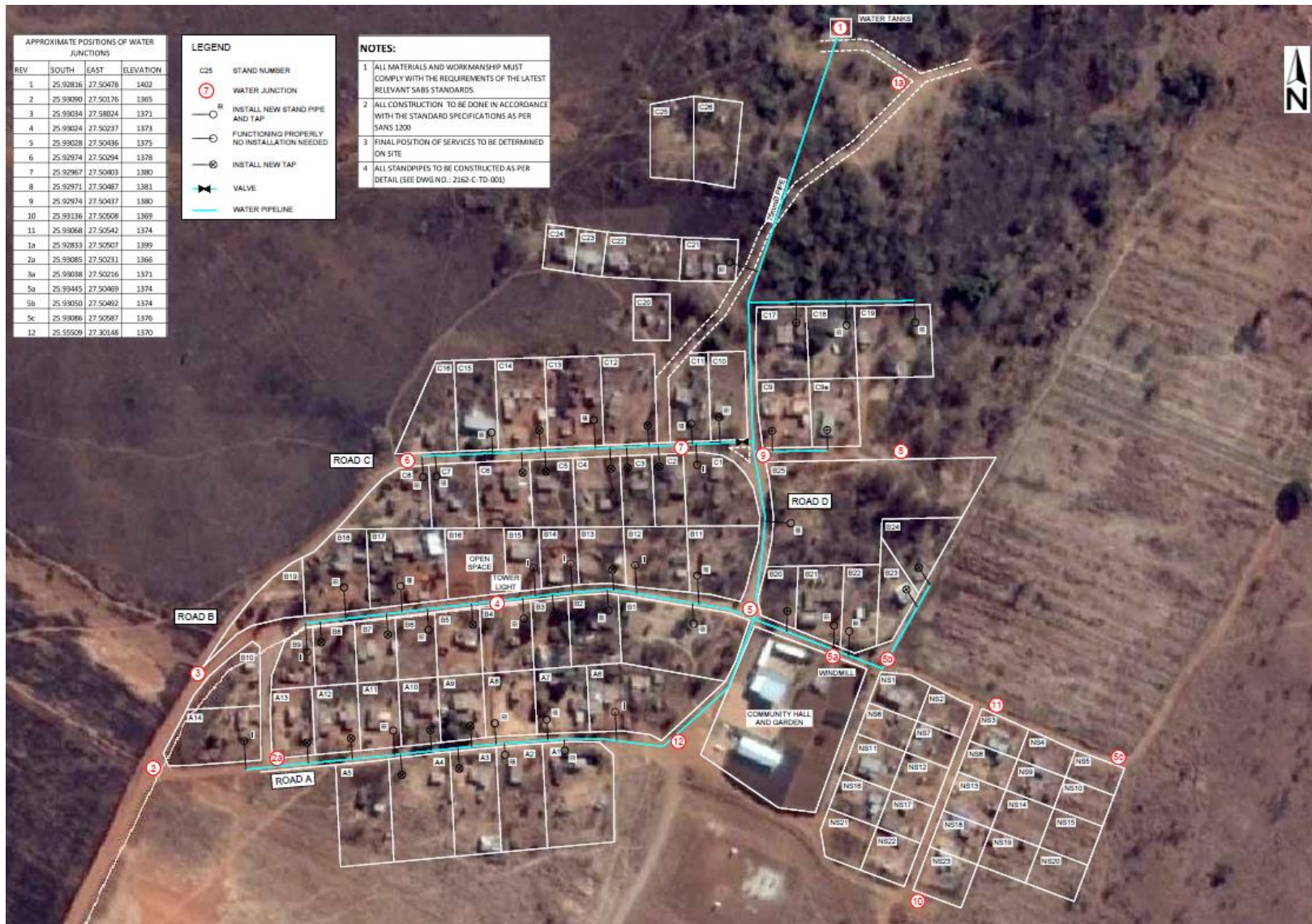
Figure 4.2 : Existing water distribution network (SFCE 2015)
