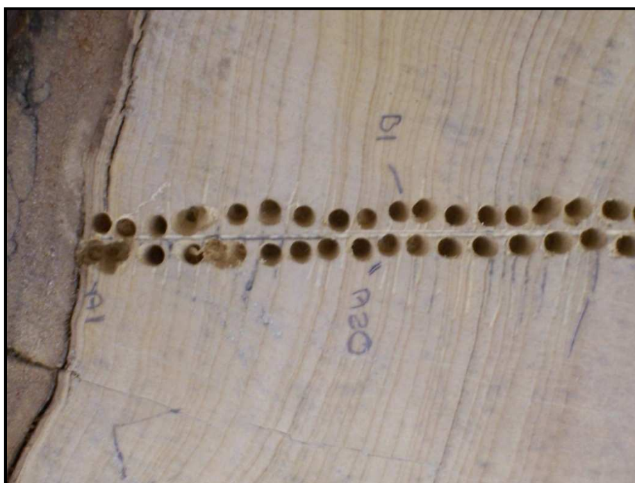
Figure A.5. Close-up view of samples drilled from Podocarpus falcatus from Baviaans Kloof, Eastern Cape. The first sample (A1) has been taken at the boundary between the bark and the first growth ring (left).
