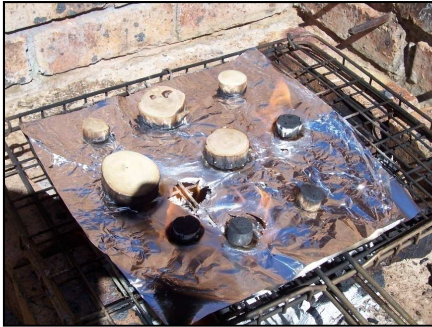
Figure A.4. Branch samples combusting under oxidising conditions.
