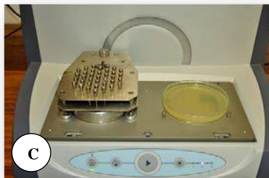
C The metal inoculators were submerged into the inoculum.
