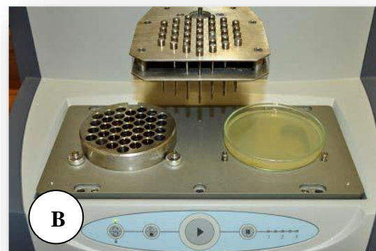
B The agar-soap plate was placed on the petri dish holder while the metal inoculators were in starting position.
