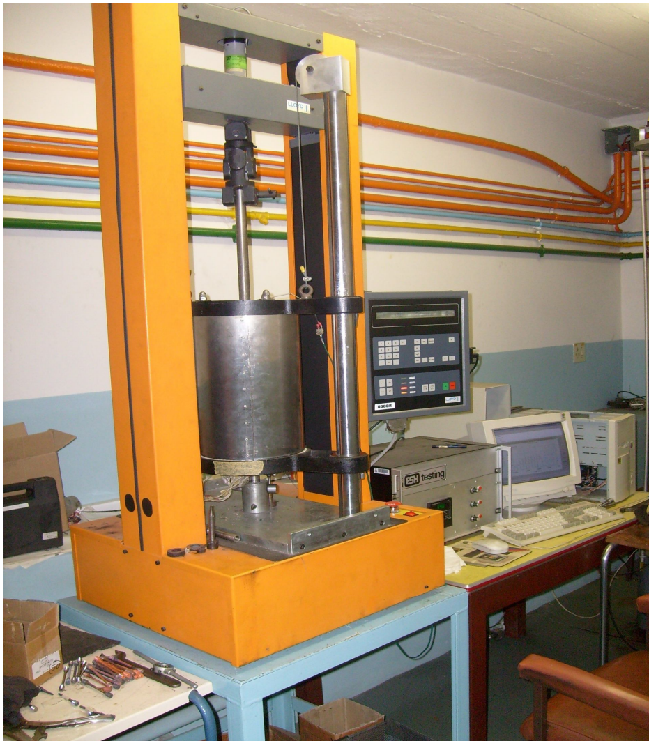
Fig. 7: Lloyd machine with auxiliary components including a desktop computer and a control panel
