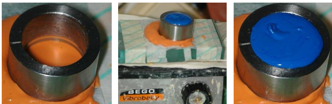
Fig. 4. Left: gypsum mould(with a lubricated interior) fitted over the alginate mould containing the set alginate; Middle: the same assembly with the gypsum poured in on top of a vibrator; Right: the filled gypsum mould waiting for complete setting of the gypsum.
