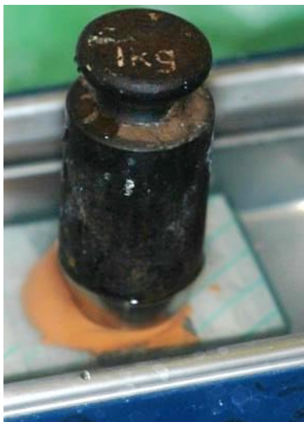
Fig. 3. The standard die placed on the alginate mould, immersed in water, and with a 1kg weight placed on the die.
