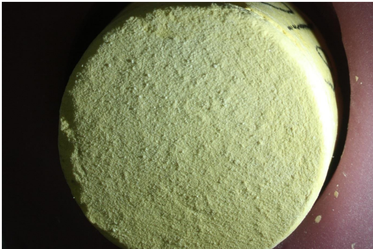
Fig. 8. This cast received a score of 4: More than 50% of the line cannot be seen properly or the line can hardly be seen at all
