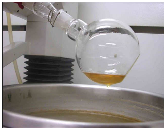
Figure 2.3: Concentrating the smoke fraction.
