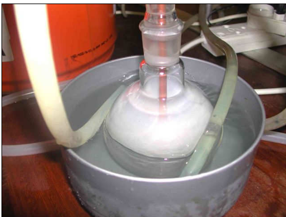
Figure 2.2: Smoke captured in hexane-methanol.
