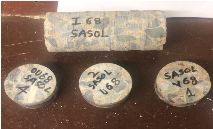
Figure 3.10: Typical 68 mm diameter core with 30 mm thick disc taken from a test structure, for DI testing at Wits concrete lab
