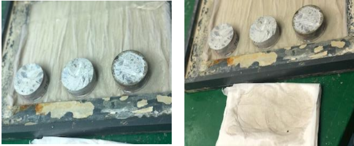
Figure 3.14: Water sorptivity testing underway at Wits University concrete lab
