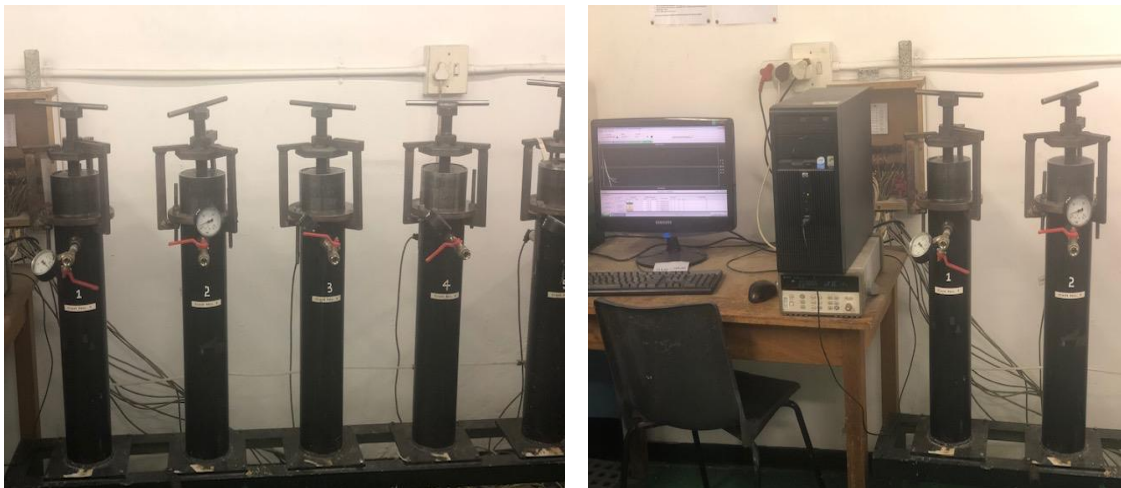
Figure 3.12: OPI apparatus and test underway at Wits University Concrete Lab
