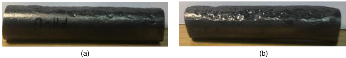
Figure 4.22: Photographs of a corroded steel bar extracted from the core sample a) U and b) S from Forest Hill reservoir are shown here
