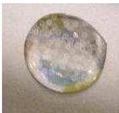
Figure 2.9 Poly-L-lysine/alginate beads in a drop of saline solution.
