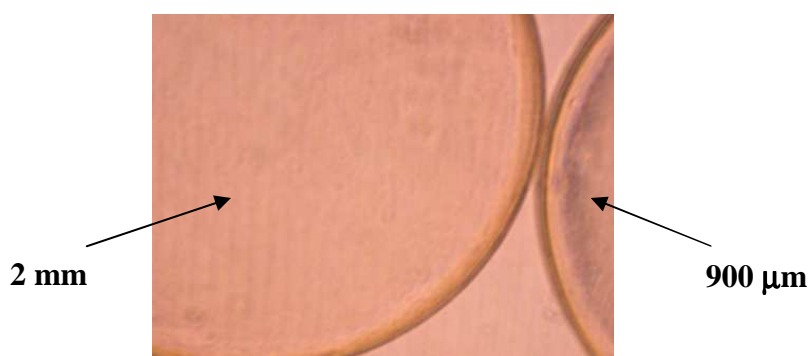
Figure 4.5. Microscopic photo of the 900 \mu\text{m} and 2 mm beads illustrating the different membrane thickness
