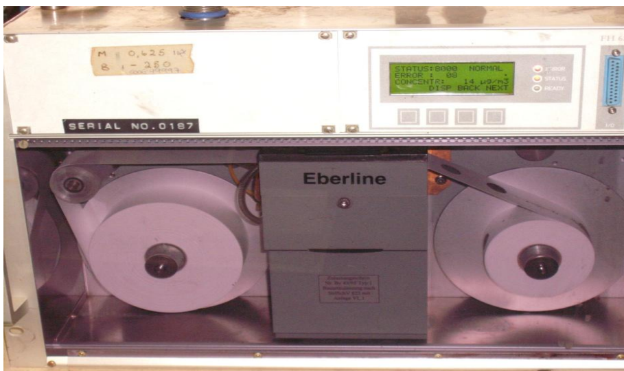
Figure 7: Eberline FH 62 I-R Beta Gauge particulate monitor, used at Leandra monitoring station for PM 10 measurements (Photo: C. Mugabo).
