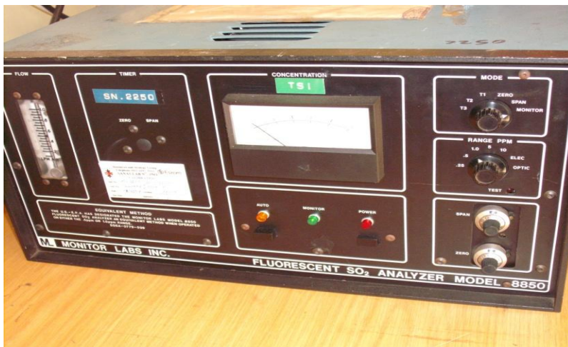
Figure 6: Monitor Labs Model 8850 Fluorescent SO 2 analyser, used at Leandra monitoring station (Photo: C.Mugabo).
