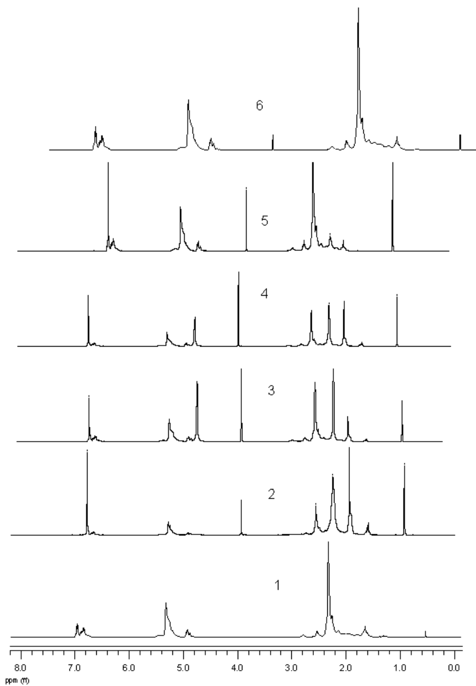
Figure 5.1: ^1\text{H} NMR of different sulphonating agents: 1= unsulphonated; 2 = fuming sulphuric acid; 3= sulphuric acid; 4 = fuming sulphuric/sulphuric acid; 5 =acetylsulphate; 6 = chlorosulphonic acid
