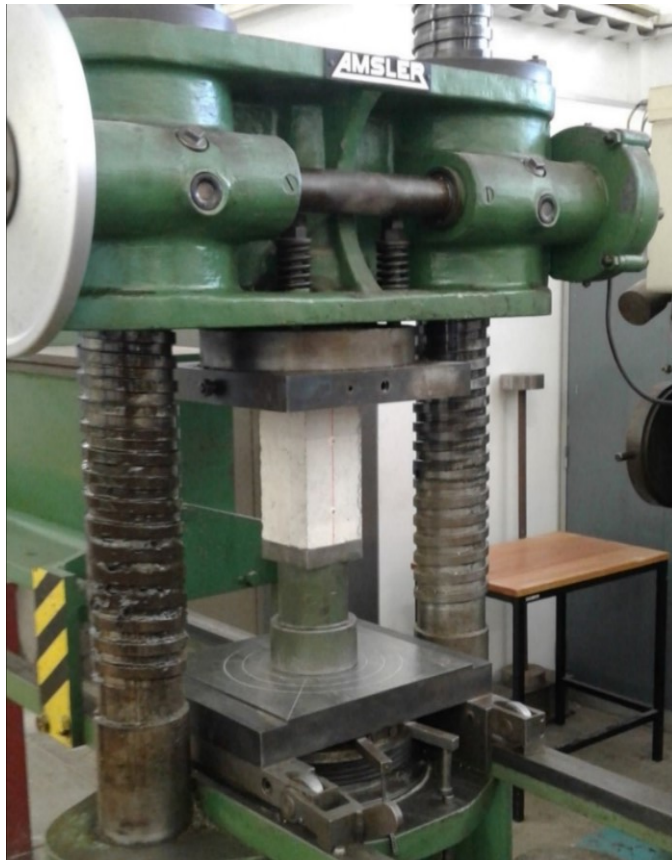
Figure 3.18: Elastic modulus specimen placed centrally in loading machine
