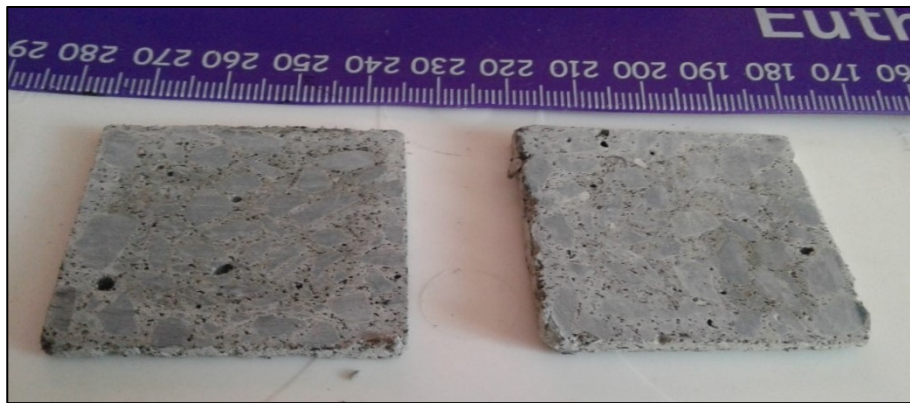
b) Fluorescent microscopy specimens ( 40 \times 40 \times 4 mm)
