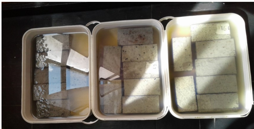
Figure 3.22: Concrete specimens immersed in ethanol with fluorescent dye
