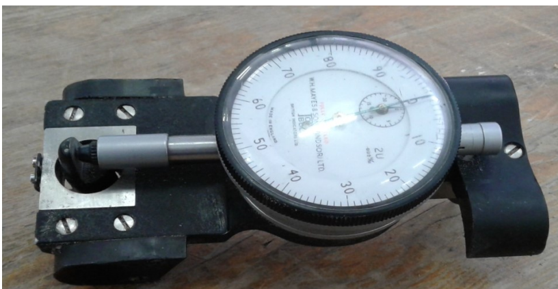
Figure 3.17: 100 mm Demec gauge (accuracy \pm 16\mu\epsilon )
