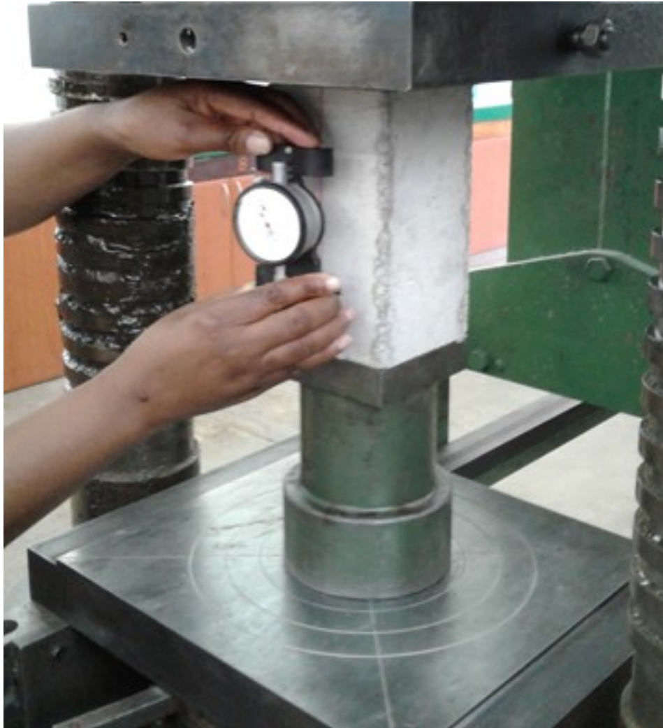
Figure 3.19: Demec gauge held in place on one face of the test specimen
