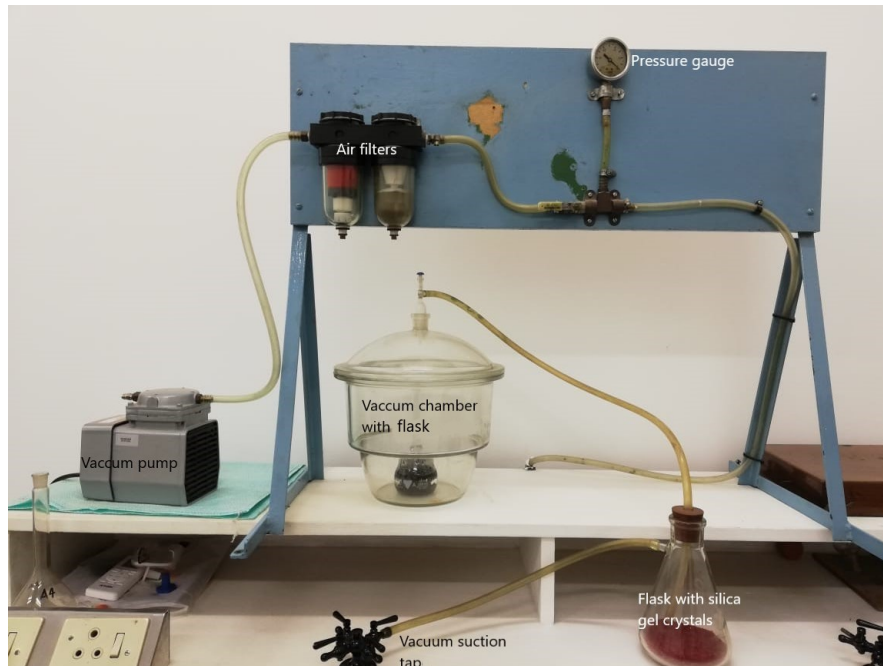
Figure A.2: Air suction apparatus arrangement
