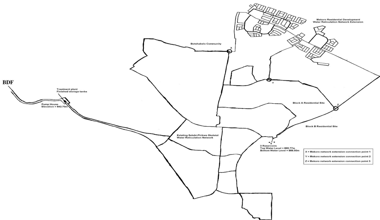
Figure 4. Skeletal layout of the existing SP WRN and proposed Mekoro, Block A and Blocks B developments.
