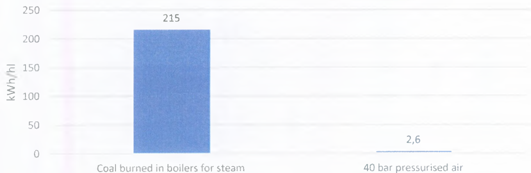
Figure 34: CED for boiler and HP compressor
