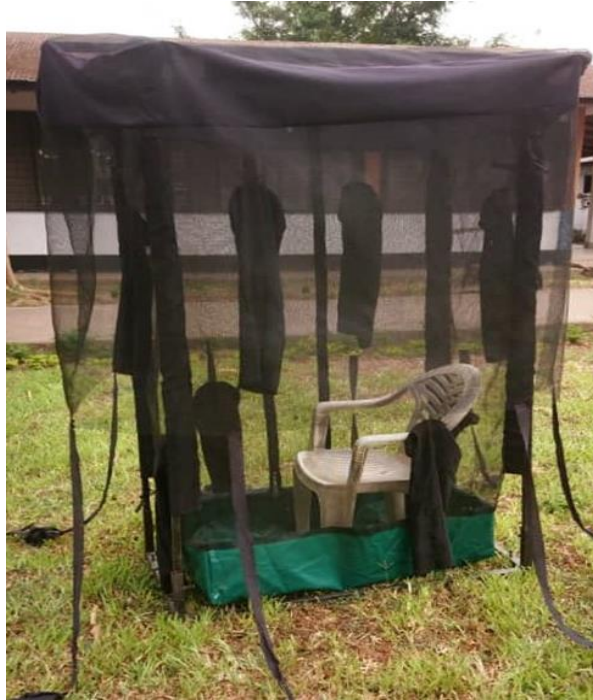
Figure 2.1: A miniaturized double-net trap (DN-Mini) that was used for comparison of indoor and outdoor host seeking mosquito densities.
