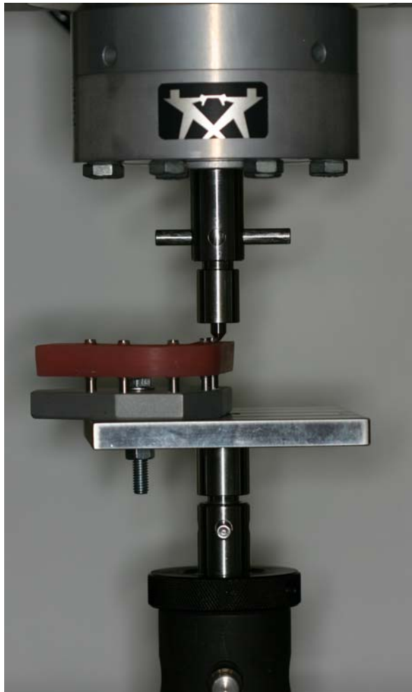
Fig 7. Platform allowing axial alignment
