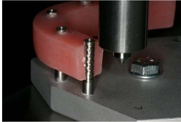
Fig 8. Fracture of non-reinforced sample
