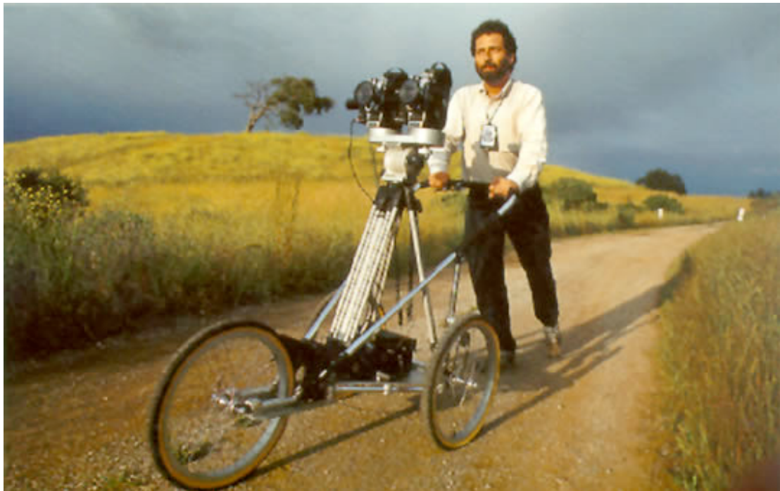
Figure 7: The “Super-Jogger” baby carriage rig used to film See Banff! footage
