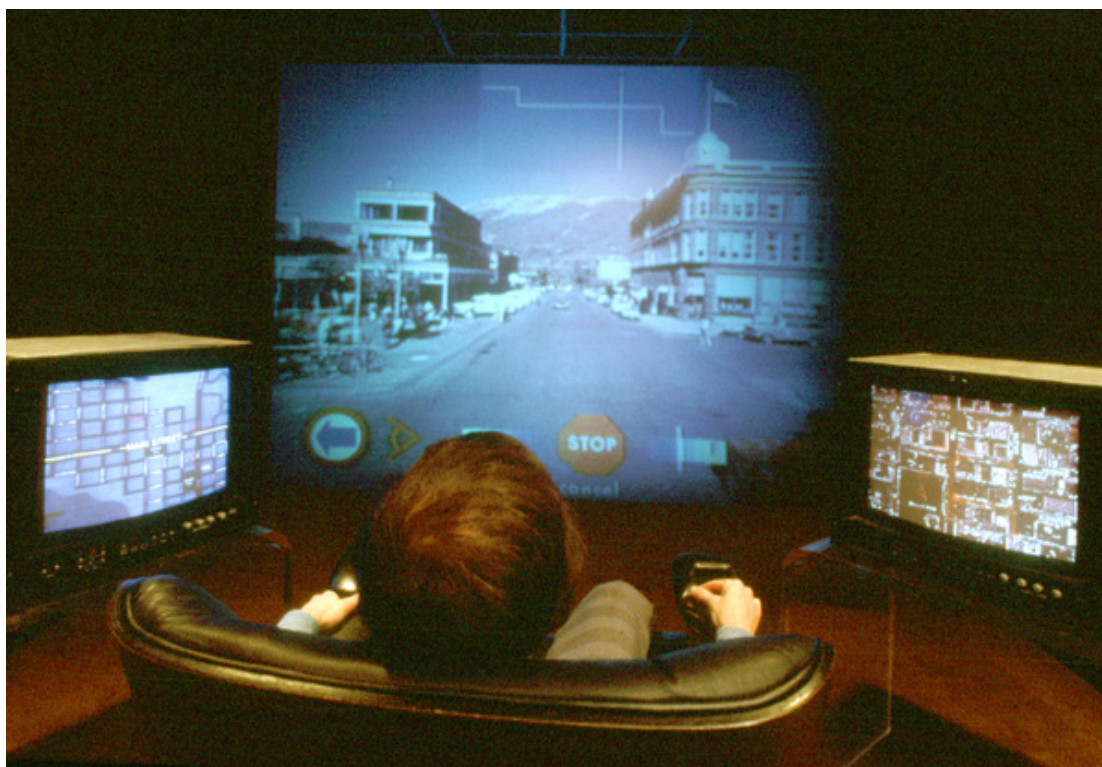
Figure 4: The Aspen Moviemap experienced in the “Media Room” at the Architecture Machine Group, MIT, c1980. The “traveler,” seated in an instrumented armchair, controls speed and direction of travel. Touch screens displaying map and aerial views allow access to additional multimedia material (Photo: Bob Mohl) (Naimark 2006).
