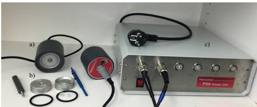
Figure 3.1: Structural components of the Hemotek ® feeding system used during blood feeding optimisation of a laboratory An. funestus colony: a = heating plate: b = reservoir, O-ring, plug and blue temperature setting device: c = power unit (Captured by M.P Zengenene at NICD).
