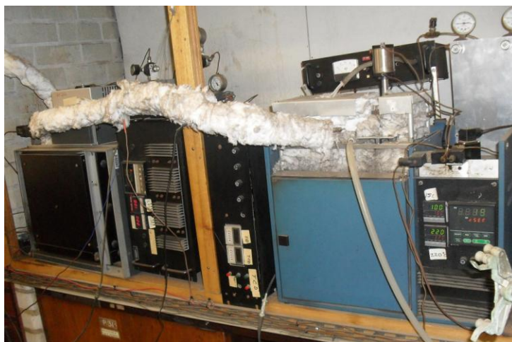
Figure 3.4 The two online GCs that were used for the analysis of gaseous products. The GC on the left is fitted with an FID detector and the one on the right is fitted with a TCD detector.
