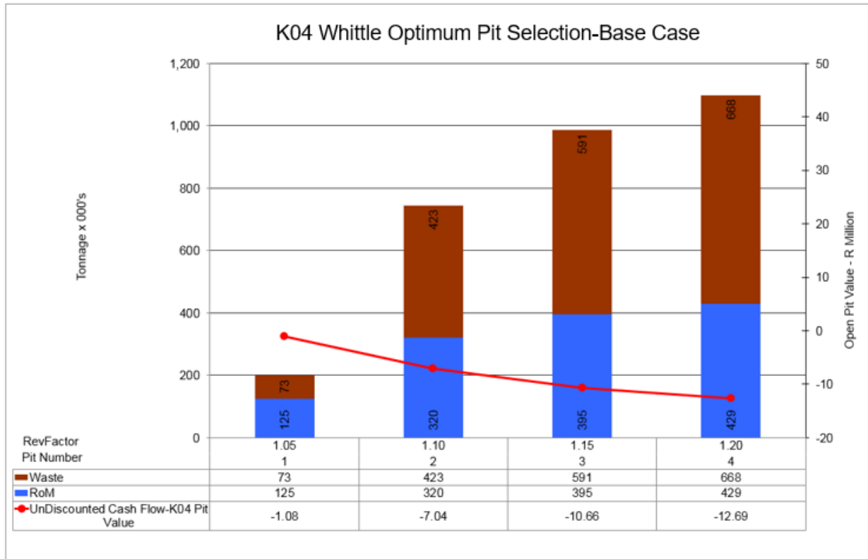
Figure 4-1: Base case pit by pit K04 optimum pit selection and discounted cash flow value.
